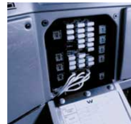
The electrical system sets the standard both for reliability and repairability, thanks to design features like these. (left) Packard Metripack 280 connectors are used extensively throughout the cab, providing an extremely positive, dependable electrical contact with little maintenance required. (middle) All wiring is heavy-gauge, neatly organized and number-coded every three inches for easiest tracing. (right) The fuse box is centrally located within the dash to allow for easy and comfortable access to fuses and circuit breakers.
