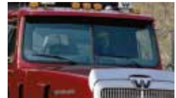
The large, laminated and curved two-piece windshield allows for excellent, panoramic visibility while minimizing repair time and cost. It features a standard bonded design, but is available with optional rubber gasket mountings in certain daycab applications.
