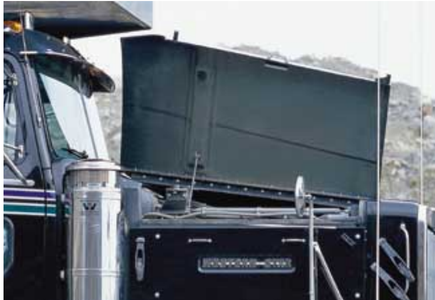
The 6900XD comes with an optional butterfly hood for quick access to inspection points and routine maintenance.
